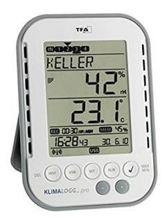
The NEW KLIMALOGG Pro temperature and humidity station can record up to 50,000 sets of data and transmit them via the wireless USB receiver (included) to your PC.
